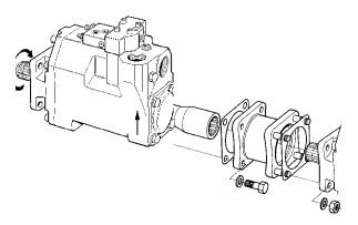
Fig. 3. Adaptor kit (P/N 379 7795) for tandem coupling.
