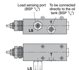
3. Basic valve setting (factory set) DO NOT TOUCH! 4. Standby pressure setting, factory set at 25 bar; (1 turn = 17 bar) LS control cross section.
