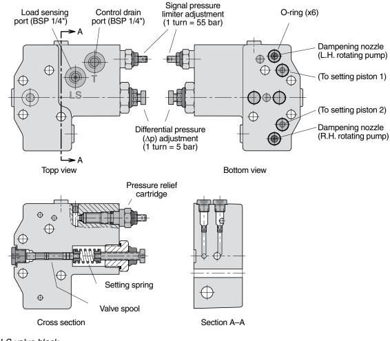
Fig. 2. LS valve block.
